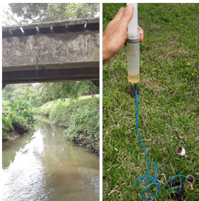
Figure 3 – Collection of water samples in the river using a piezometer.
