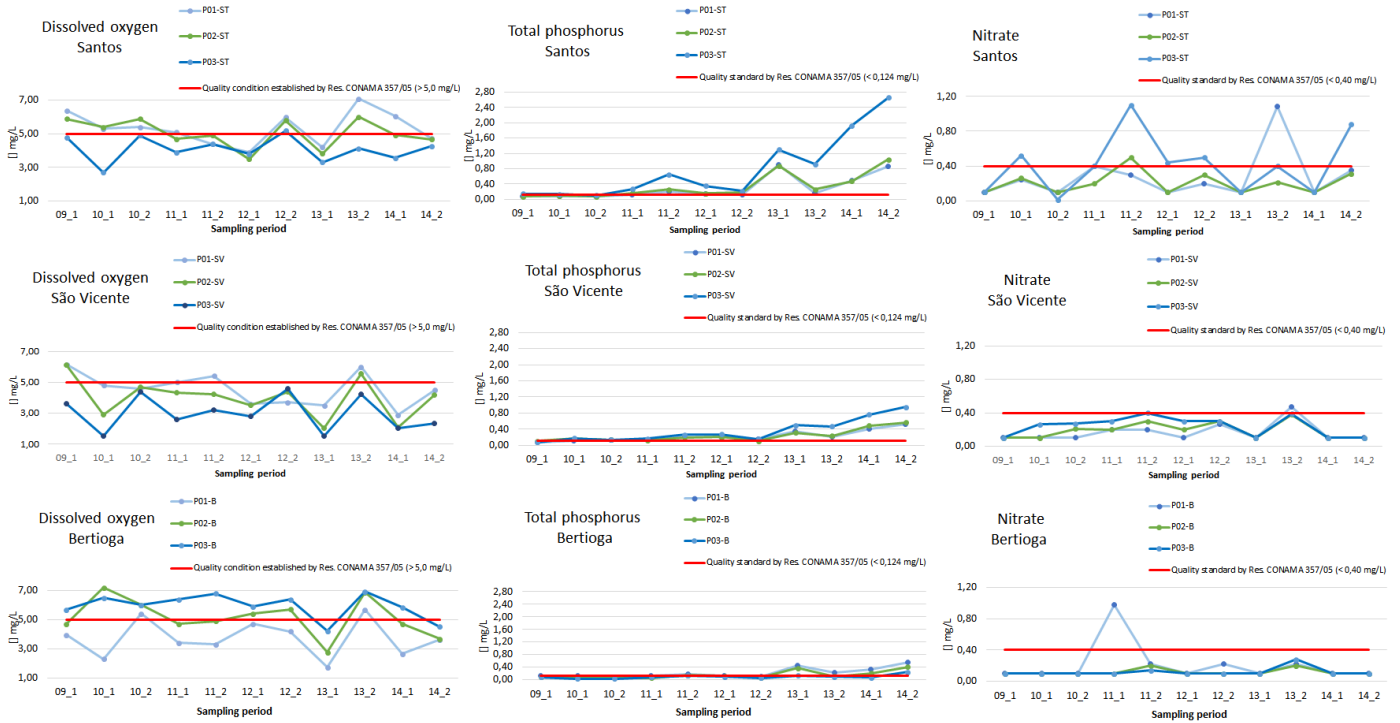
Figure 3 – Results of dissolved oxygen, total phosphorus, and nitrate concentrations in water samples during the 11 semi-annual sampling campaigns, between 2009 and 2014.
