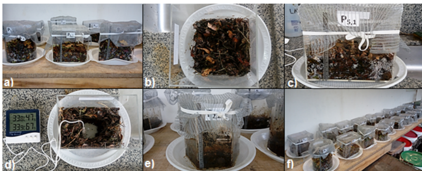
Figure 4 – Laboratory bench test monitoring. (A and F) View of the experiment installed on a laboratory bench; (B) internal view of the prototype in operation; (C and E) front view of prototypes and detail of the sanitary control screen; (D) monitoring of moisture and temperature using a thermo-hygrometer.
