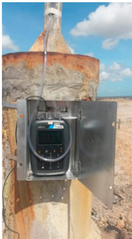
**Figure 1 – Gas measurement in a drain of the Sanitary Landfill in Caucaia, Ceará, Brazil.**
