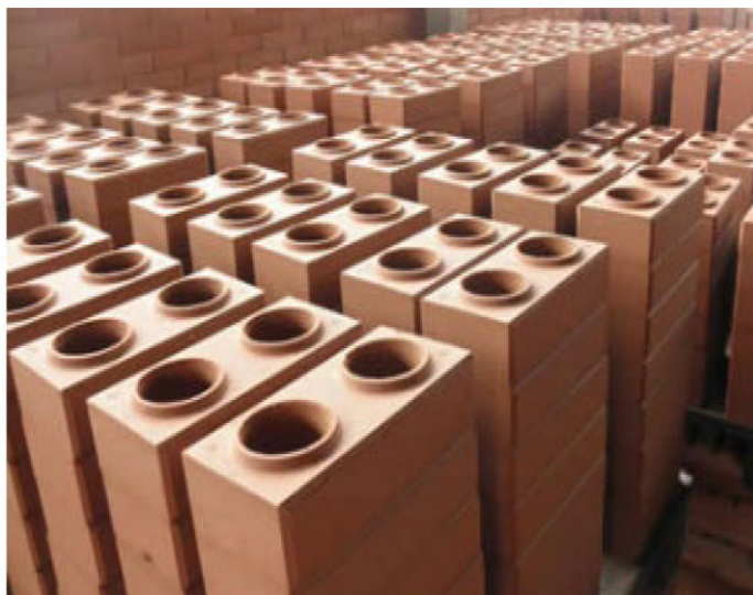
Figure 1 – Soil-cement blocks. (A) Holes in soil-cement blocks. (B) Ducts in soil-cement blocks. Source: Eco Máquinas.
